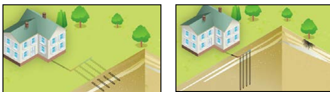
Fig. 6 – Geothermal system installed under the ground. A) horizontal, and B) vertical construction
